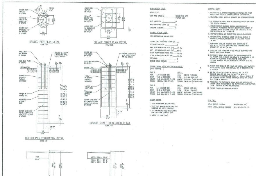
TRAFFIC SIGNAL MAST SCHEMATIC TRAFFIC SIGNAL MAST SCHEMATIC DRAWING NOT TO BE SCALED 2000 M DN DRIGINAL DRAVING CASE 1 CASE 2, 3 & 4 DRAWING NOT TO BE SCALED. ALL DIMENSIONS ARE IN MILLIMETRES UNLESS OTHERWISE SHOWN. DATE DRAWN BY DRAWING No. DATE MINSITRY OF WORKS AND TRANSPORT POK 2010/07/13 S04 ESIGNED BY DRI, SCALE: TRAFFIC SIGNAL MAST ARM SHEET No. WBK AS SHOWN FOUNDATION DETAILS 28
